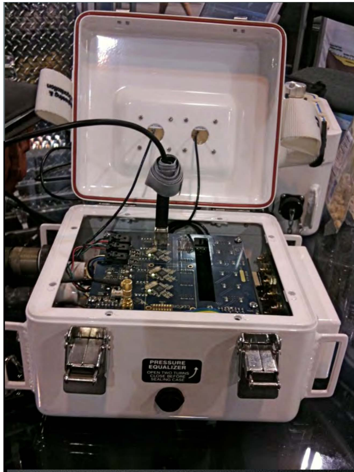
Figure 5-3 OSU/Zonge High Definition Wideband EM Receiver for Electric and Magnetic Fields
