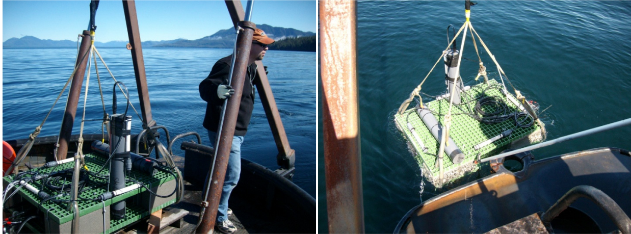
Figure 7 - Deployment of probe assembly at in-situ test site
