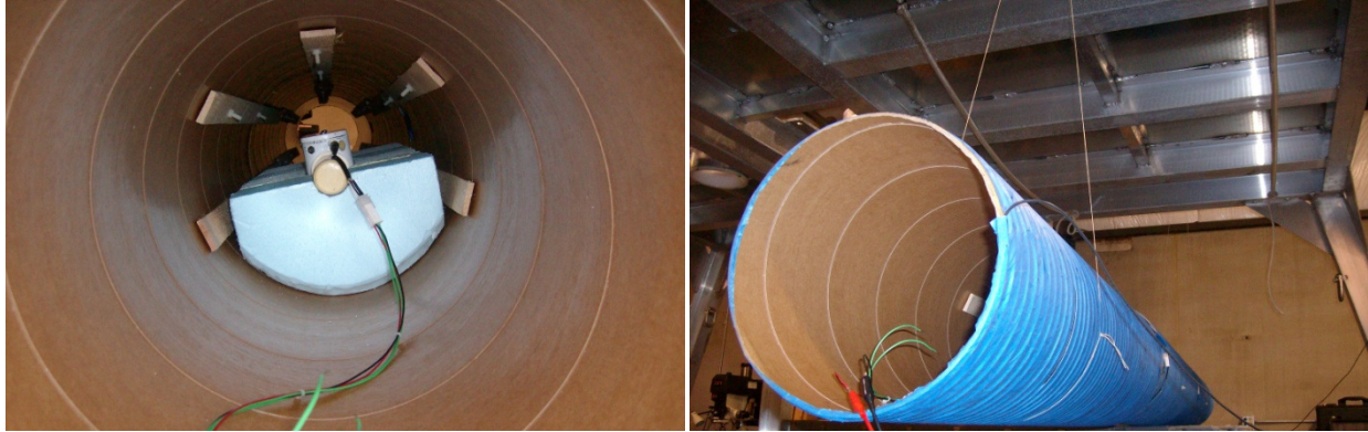
Figure 5 - Magnetic sensor undergoing magnetic calibration
