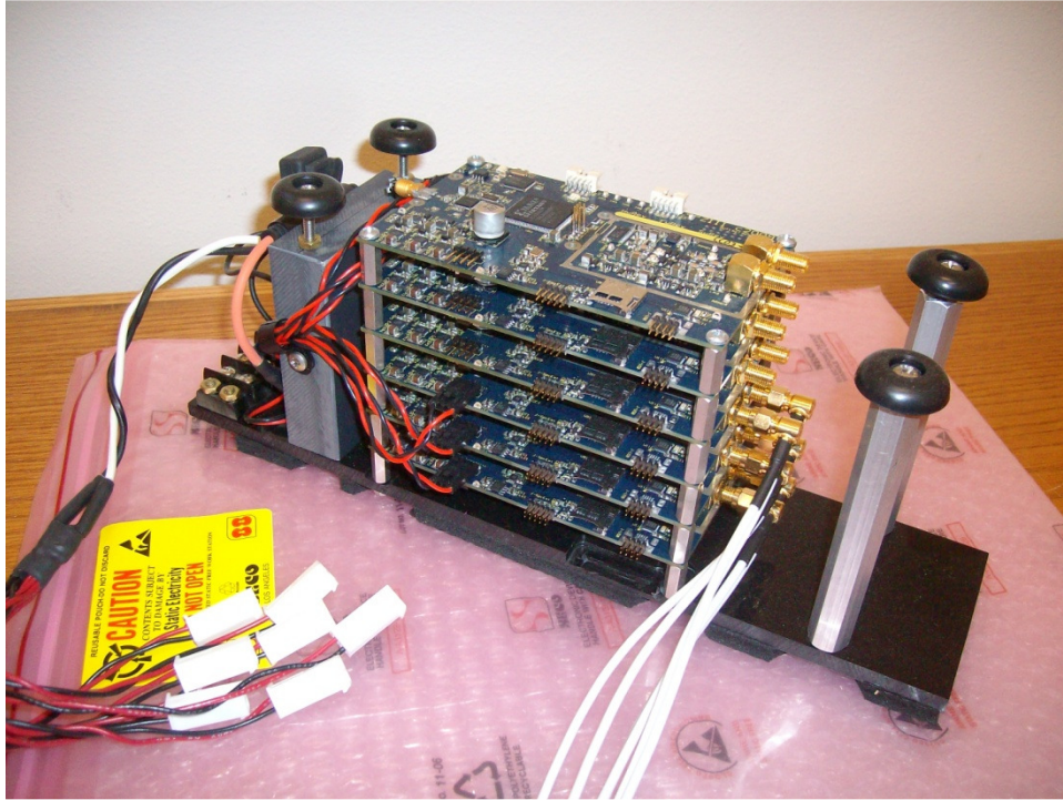
Figure 4 - Six-channel data recorder assembly 'stack'
