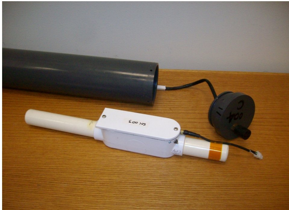
Figure 2 - Uniaxial magnetic field sensor, shown with non-metallic pressure vessel
