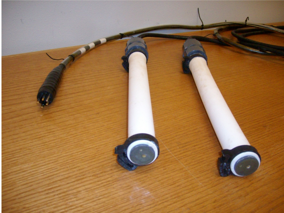
Figure 3 - Electric field probes and wet-mate interconnect cable
