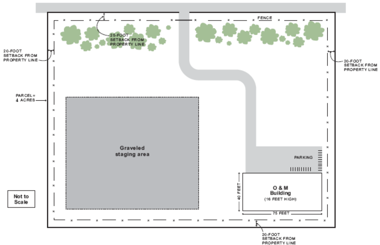
Figure 2-13 Typical O&M Facility Layout
