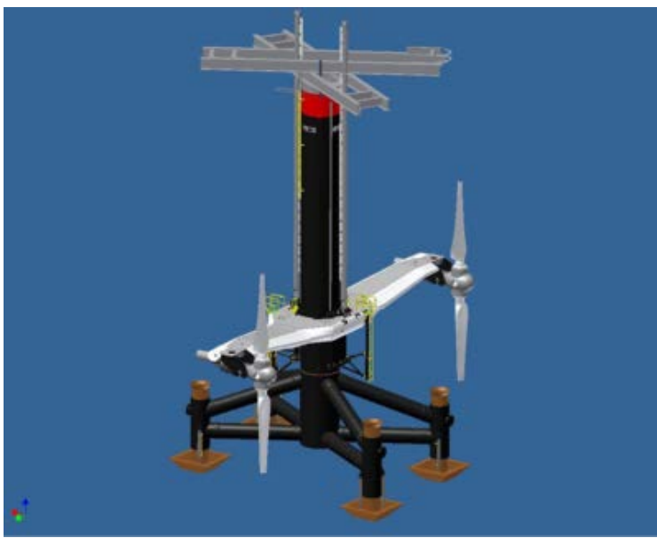
Siemens/MCT Foundation Arrangement
