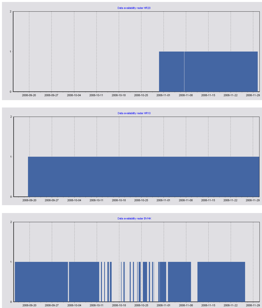
Figure 4-4. Data coverage from the three radars. All three radars were running with 24 hr coverage. Unfortunately, due to weather and logistical constraints the installation of the HR2 radar had to be postponed until 27 October, while the installation at Blåvands Huk was finalised 16 September and at HR1 at the 19 September. However, due to the coverage from HR1 of the area between HR1 and HR2 OWFs the major part of the waterbird migration between the two wind farms could be covered until the end of the migration in late November. The coverage at Blåvands Huk was broken by shorter drop-outs between 11 and 28 October. The reason for these drop-outs was the fact that the computer equipment was installed in the same room that was used by the army for different exercises, and the various army personnel accidentally switched off the power every now and then.
