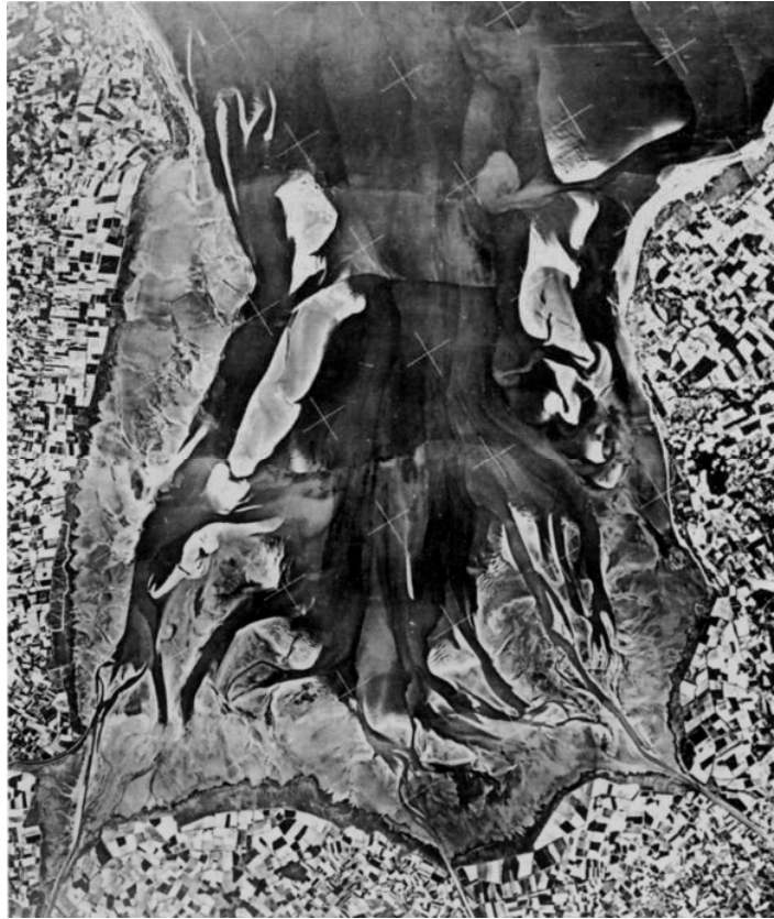
Fig. 16 Aerial photograph of the Wash showing wide estuary sand banks. The net sand transport into the estuary results in the sand banks widening once they reach sea level. From G. Evans.
