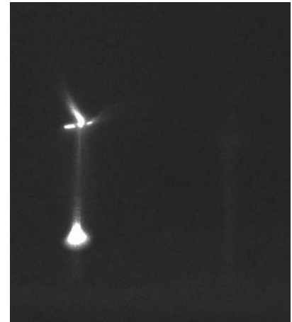
A wind turbine is dimly lit with flickering ultraviolet (UV) light and imaged by using a video camera sensitive to UV light. Image from video clip by Paul Cryan, U.S. Geological Survey.
