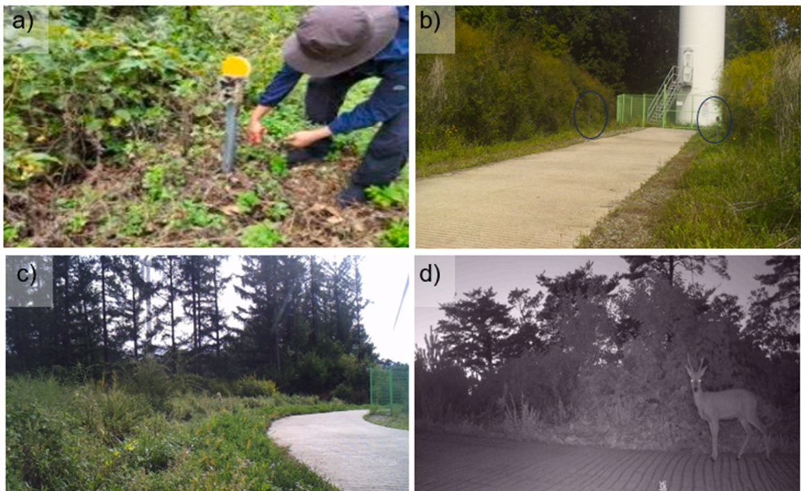
Fig. 2. Camera installation, orientation, and animal detection in survey area a) Camera installation and camera height, b) Cameras installed near to wind turbine positioning to capture forward and backward sites, c) Camera captured wide road in curve section, d) Wildlife (roe deer) captured on camera while moving along the road.
