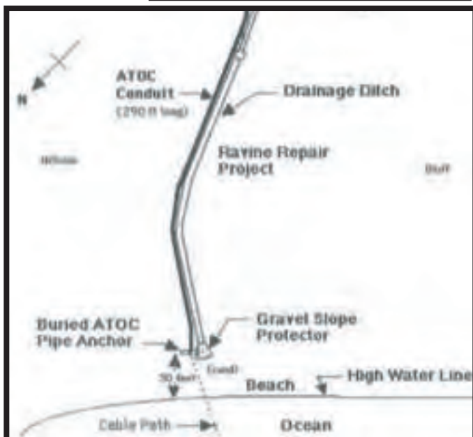
Figure 22: Photographs and diagram of the beach near Pillar Point where the ATOC/Pioneer Seamount cable comes on shore. North is to the left in all photographs. A: Photograph showing the relative positions of the drainage ditch and the submarine cable exposed on the beach taken in July 2003. B: Photograph showing a close-up of the cable taken in October 2002. C: Photograph showing a close-up of the cable taken in July 2003. Note that a cement block is seen in the more recent photograph. Also note that more of the cable is exposed behind the deadman anchor in the more recent photo and that the cliff face has retreated. D: Diagram showing the location of the ATOC/Pioneer Seamount cable buried anchor relative to the drainage ditch (University of Washington 1995).
