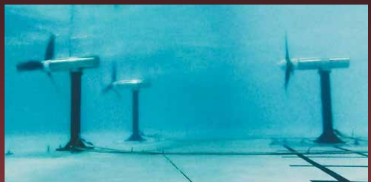
Three CMERG turbines under test in Flowave (EPSRC DyLoTTA project with Strathclyde University)
