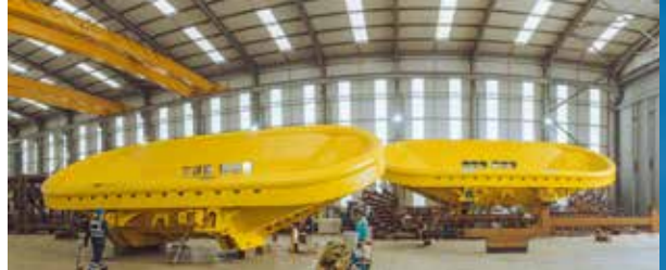
Two of the four 15 meter long cell modules that will be covered in a flexible rubber membrane and fixed to the 75 meter long demonstrator device
