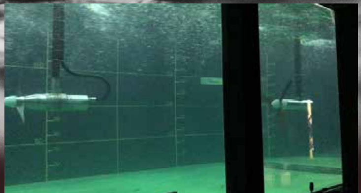
Effects of Wake-current interaction on a downstream turbine. Testing using two CMERG turbines in IFREMER flume (funded by NRN Bangor led project, EPSRC DyLoTTA and EPSRC IAA)
