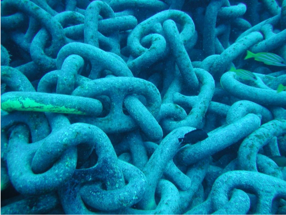
Figure 8. Ballast chain in chain locker in early 2004. Note the minimal fouling
