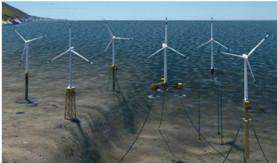
U.S. offshore wind projects are developing a variety of different foundations suited to unique conditions at each site. Illustration by Josh Bauer, National Renewable Energy Laboratory (NREL)
