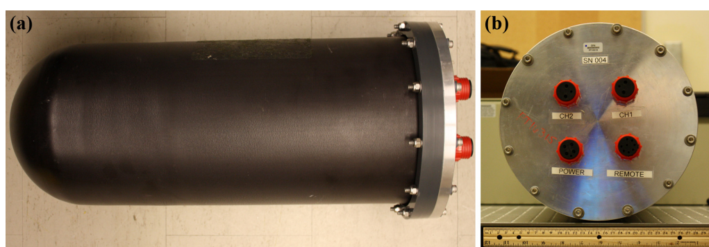
Figure 5. Submersible version of the Underwater Sound Recorder. (a) PREVCO submersible housing; (b) external waterproof connections.
