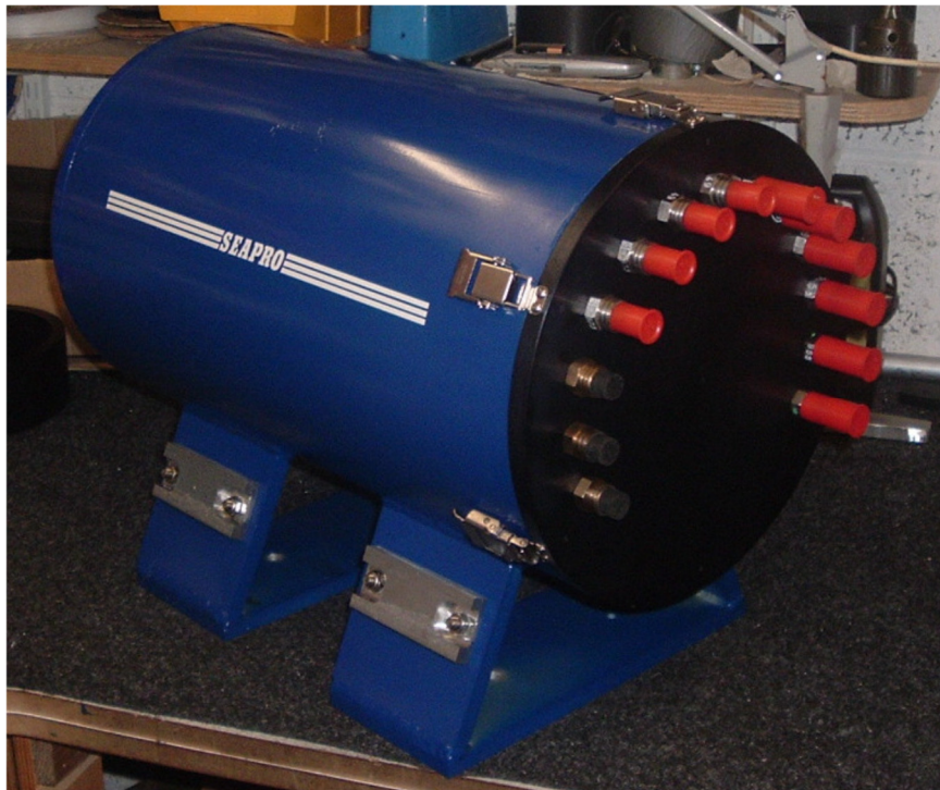
Figure 11: Example of the TSS Junction Box
