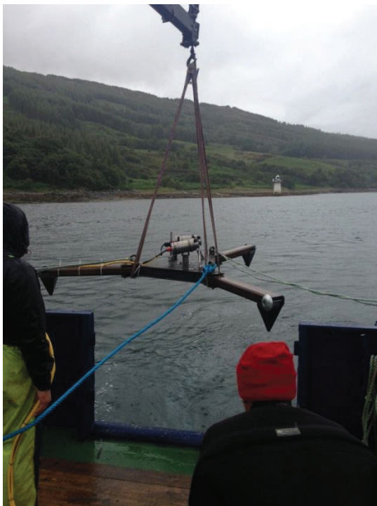
Figure 4: Hi Current Underwater Platform (HiCUP) with dual sonar configuration being deployed in Kyle Rhea.
