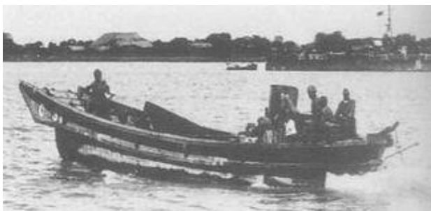
Figure 1. The Daihatsu Class or 14m landing craft used by the Japanese during WWII. (Obtained from World War II Database. Available online. URL: http://ww2db.com . Accessed on January 25, 2013).
