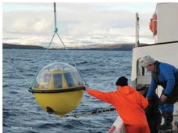
Figure 4. TRIAXYS™ Directional Wave Buoy with ADCP Launch.
