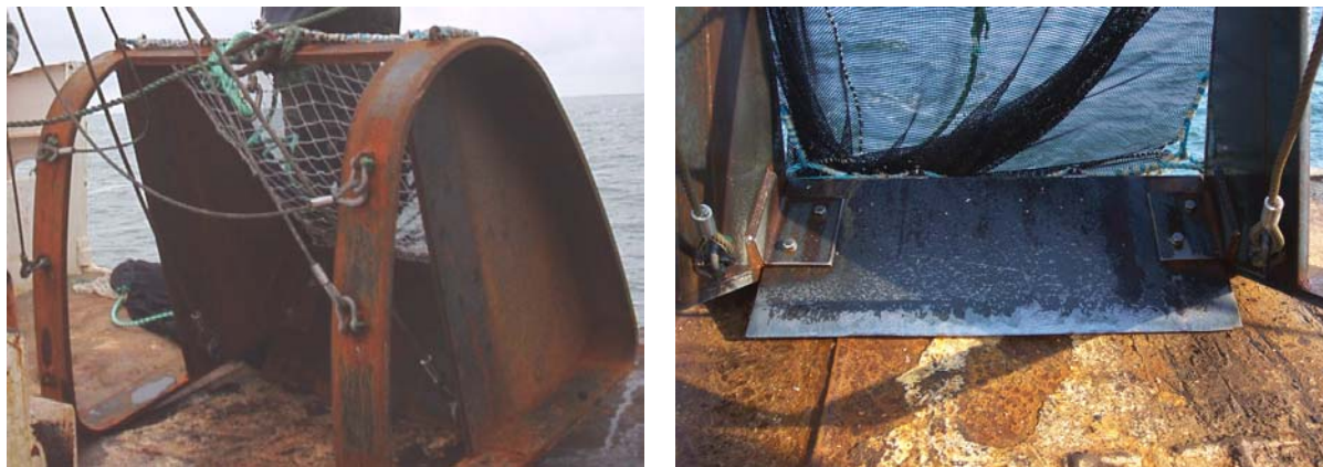
Figure 4. Dredge with nets attached (left). Detail of cutting plate (right) showing wear (note: net partly removed)
