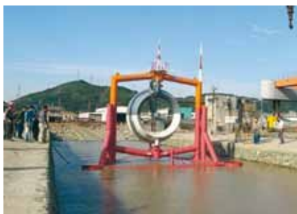
10 kW horizontal-axis tidal current prototype
