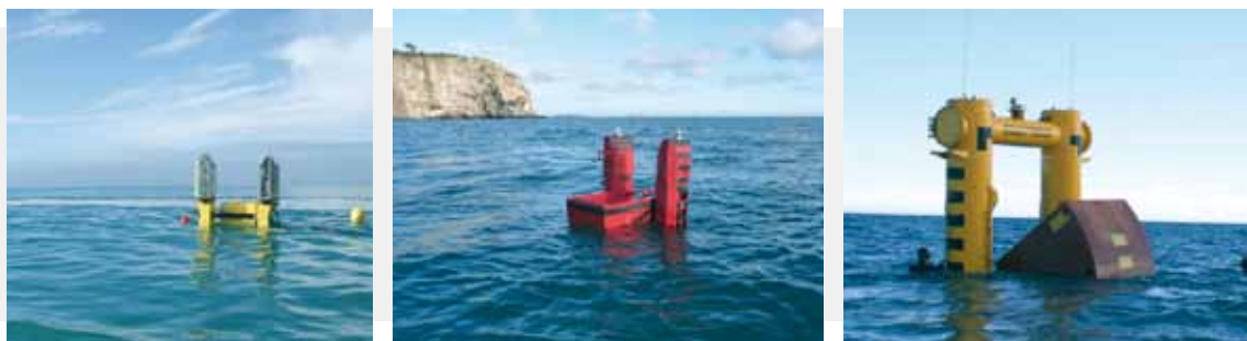
Figure 1: a) WET-NZ’s 1:5-scale 2 kW proof-of-concept device (2006-2008)
