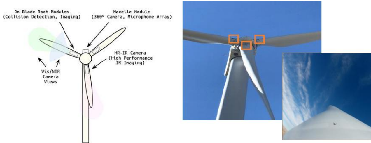
Figure 15 The wind turbine sensor array unit installed at an onshore wind farm in Boulder, Colorado (images taken from Albertani et al., 2021a)
