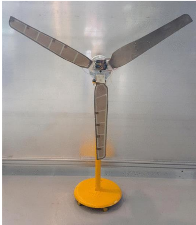
Figure 9 Turbine blades coated with 0-3 piezoelectric composite sensors (image taken from Kang and Kang, 2017)
