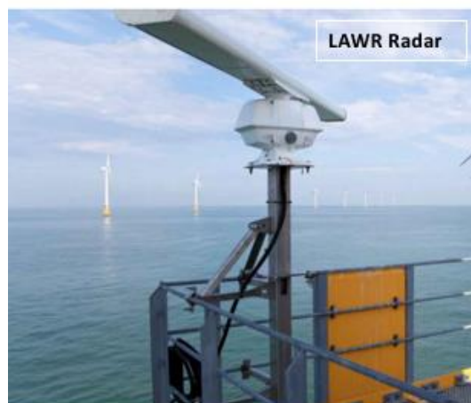
Figure 3 LAWR 25 Radar installed on turbine G05 at Thanet offshore wind farm (image taken from Skov et al., 2018)
