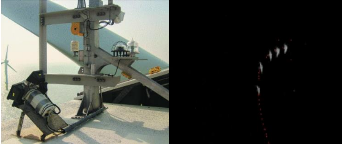
Figure 7 (left) Image of VARS installed on the nacelle of a turbine within the Alpha Ventus wind farm. (right) thermal video sequence of a bird recorded near the turbine (images taken from Hill et al., 2014)
