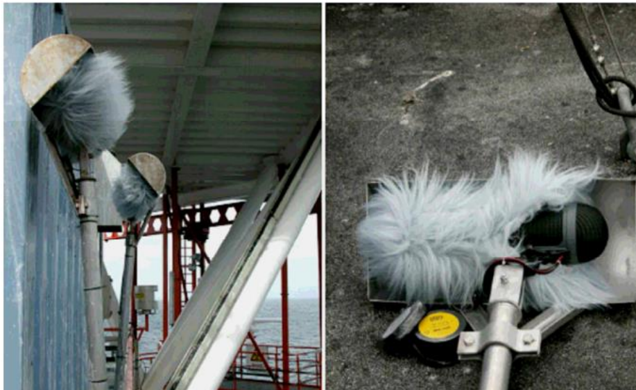
Figure 8 Microphone (and bat detector) with windshield and microphone muff installed at FINO1 near the Alpha Ventus wind farm (image taken from Hill and Hüppop, 2009)
