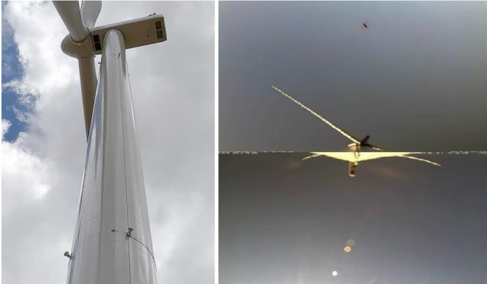
Figure 13 DT-Bird system, camera field of view and recorded detection (images taken from DT-Bird website)
