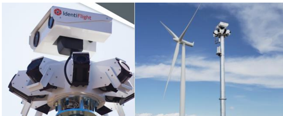
Figure 16 The IdentiFlight system (image taken from IdentiFlight website)
