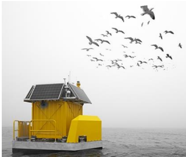
Figure 22 Fly'rsea floating radar system (image taken from Akrocean website)
