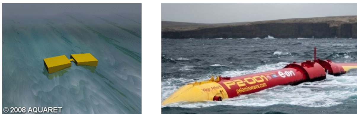
Figure 11. Left Panel: schematic of wave attenuator. Right Panel: the Pelamis wave device at EMEC, Orkney (EMEC 2014)
