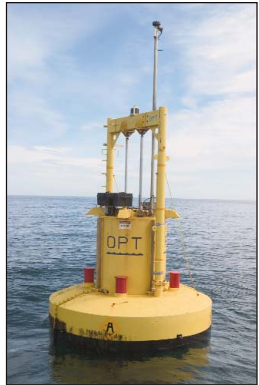
Figure 3. Photograph of PowerBouy® courtesy of Ocean Power Technologies, Inc.
