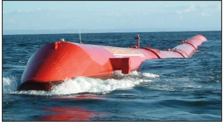
Figure 2. Photograph of the Pelamis wave power generator courtesy of Pelamis Wave Power.
