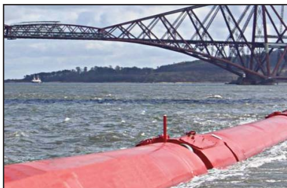
Photograph of the Pelamis wave power generator courtesy of Pelamis Wave Power.
