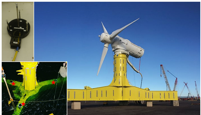
FIGURE 2 A horizontal-axis tidal turbine similar to the AR1500 turbine in the current study. (Inset; top) one hydrophone cluster. (Inset; bottom) AR1500 during installation. The position of each hydrophone cluster on the turbine support structure is indicated by a red star. Turbine images courtesy of SIMEC Atlantis Energy
