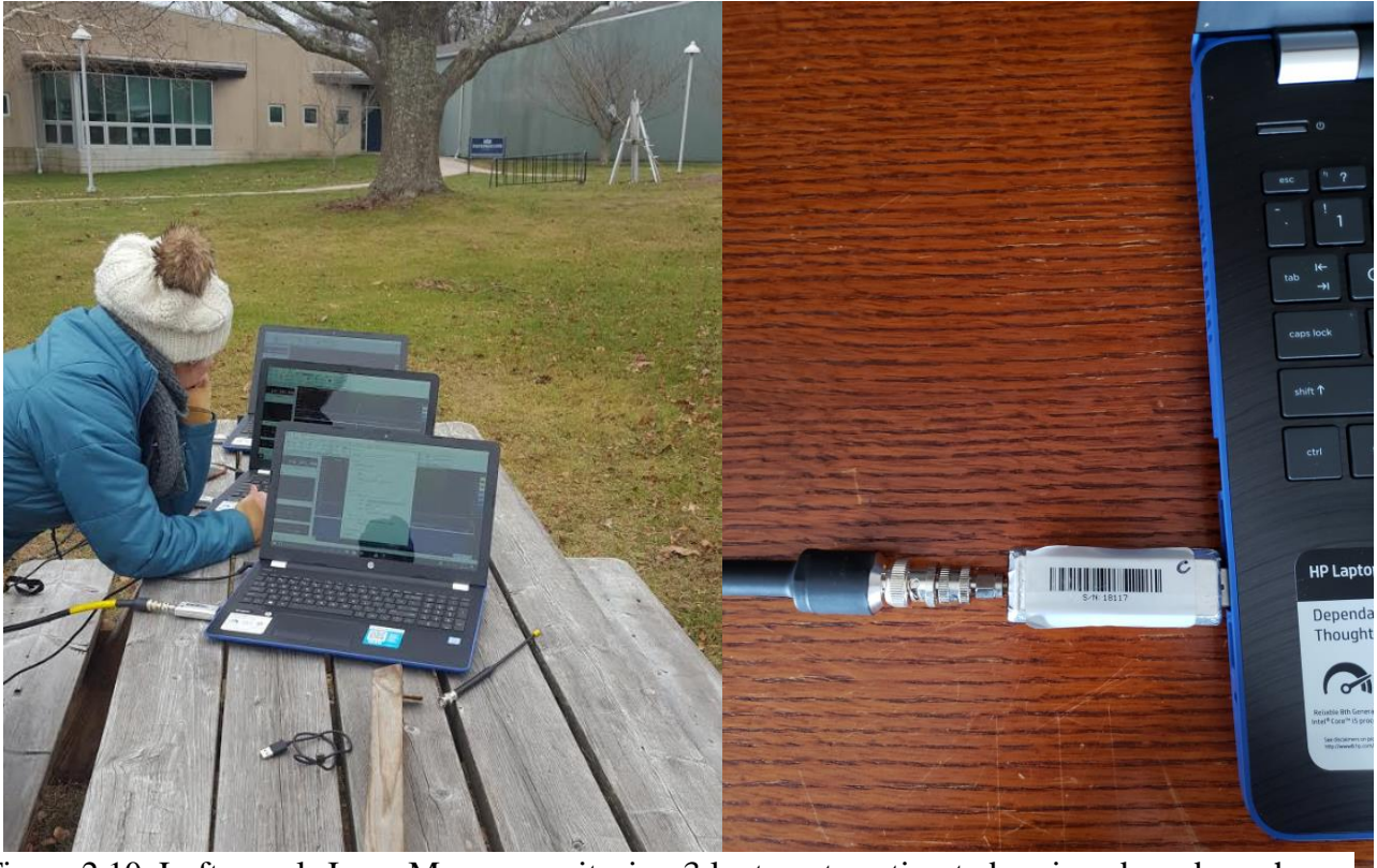
Figure 2.10. Left panel: Jesse Moore monitoring 3 laptops to estimate bearings based on phase delays, Right panel: coaxial cable connected each 6.4 m omnidirectional antenna to a FUNCube Dongle to convert the analog signals to digital for the SDR software.
