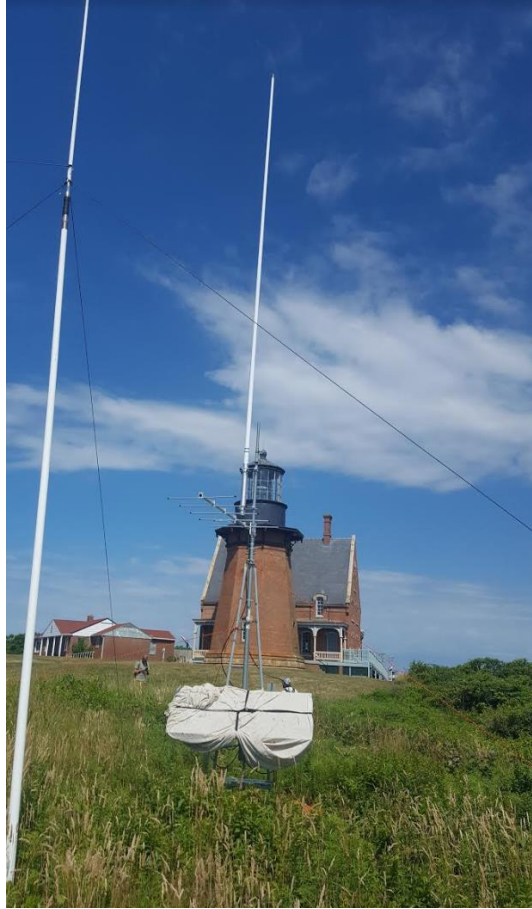
Figure 1.12. Tower being constructed for the 2018 field season at Southeast Lighthouse. Tower was built on 4 m tall pop-mast and included 1 5-element 8-dB Yagi antenna and one 6.4 m tall 10-dB omnidirectional antenna. The lighthouse was north of the tower array and another omnidirectional antenna for another project is in the foreground on the left. The solar panel was covered as the array was not operational when this photo was taken.
