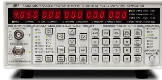
Figure 2.12. SG 380 series Rf signal generator used generate ultra-high frequency resolution ( 1 \mu\text{Hz} ) used a precise calibration source generator with rubidium timebase.
