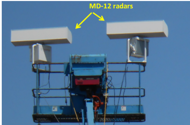
Figure 5. Photograph of MD-12 Doppler radars being used on the Eagle Take project.
