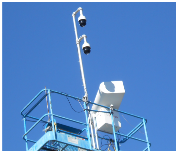
Figure 6. Photograph of two Axis A6115-E surveillance cameras that are used for tracking airborne targets.
