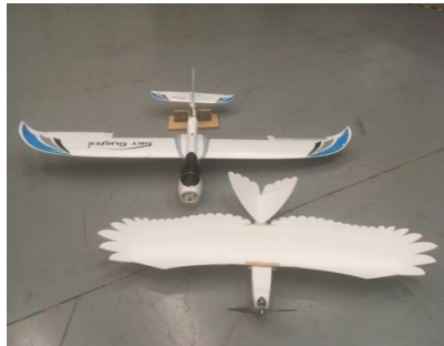
Operational Eagle surrogate drones at Bedford NH
