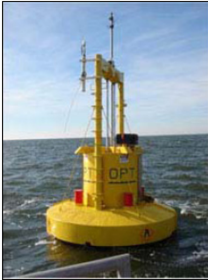
Figure 25 - OPT PowerBuoy Device
