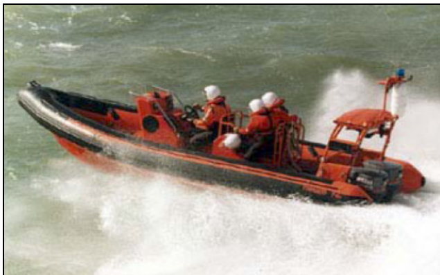
Figure 10 - Typical Rigid Inflatable Boat (RIB)
