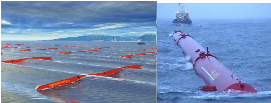
Figure 20 - Pelamis Wave Power Devices
