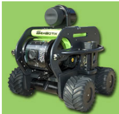
Figure 12 - Seabotix Crawler ROV
