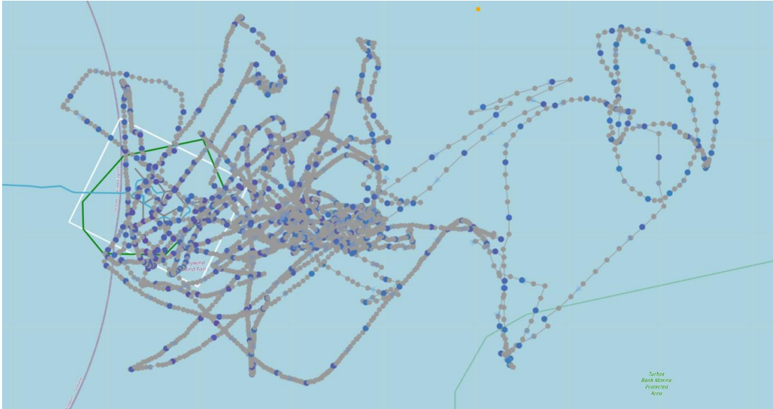
Figure 4 Sampling tracks on site (June 25 th to July 23 rd ). Grey dots are GPS positions, blue dots represent EK80 samples, every 15 min and every hour respectively within and outside of the operation area (white rectangle).
