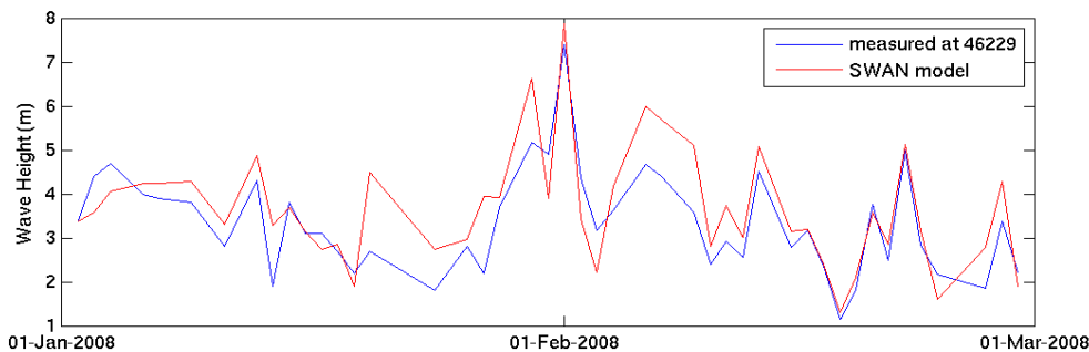
Figure D4: Comparison between predicted (red) and observed (blue) wave height at NDBC buoy 46229 over 2 months of simulations.
