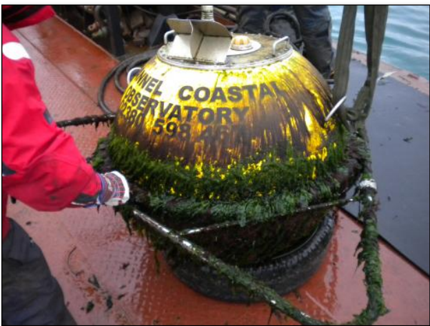
Fig. 4. Heavily fouled directional waverider buoy [38].
