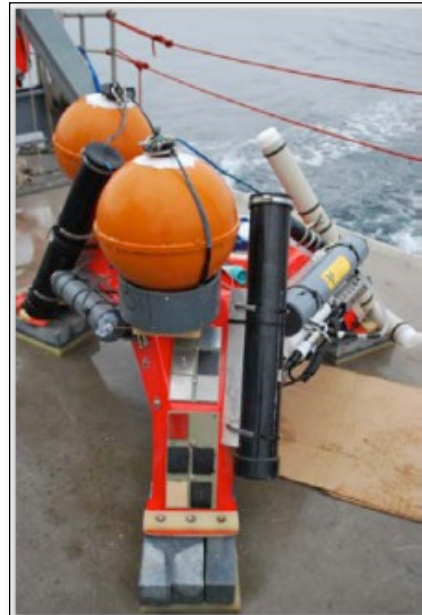
Fig. 6. Material samples attached to instrumentation tripod [10].
