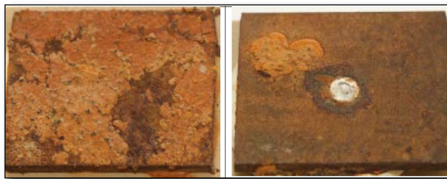
Fig. 12. Structural steel coupon corrosion [10].
