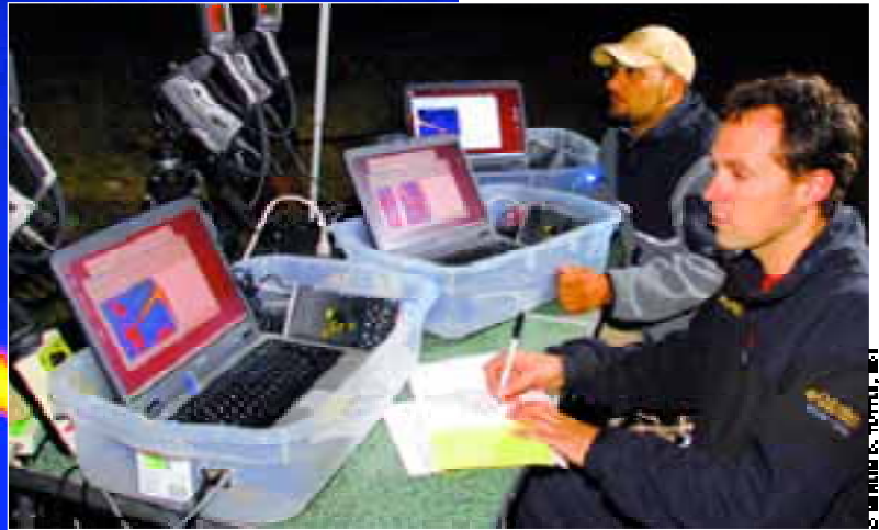
Jason Horn (right) and Roger Rodriguez monitor thermal images being recorded at wind-energy turbines of the Mountaineer, West Virginia, facility. The image at left shows a bat approaching a potentially lethal turbine blade.
