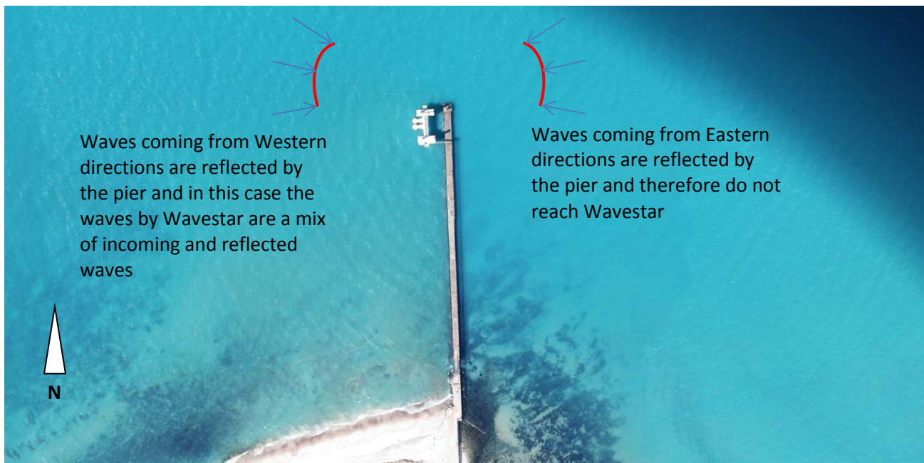
Figure 13: Position of Wavestar by Roshage with sketch of waves from Eastern and Western directions.
