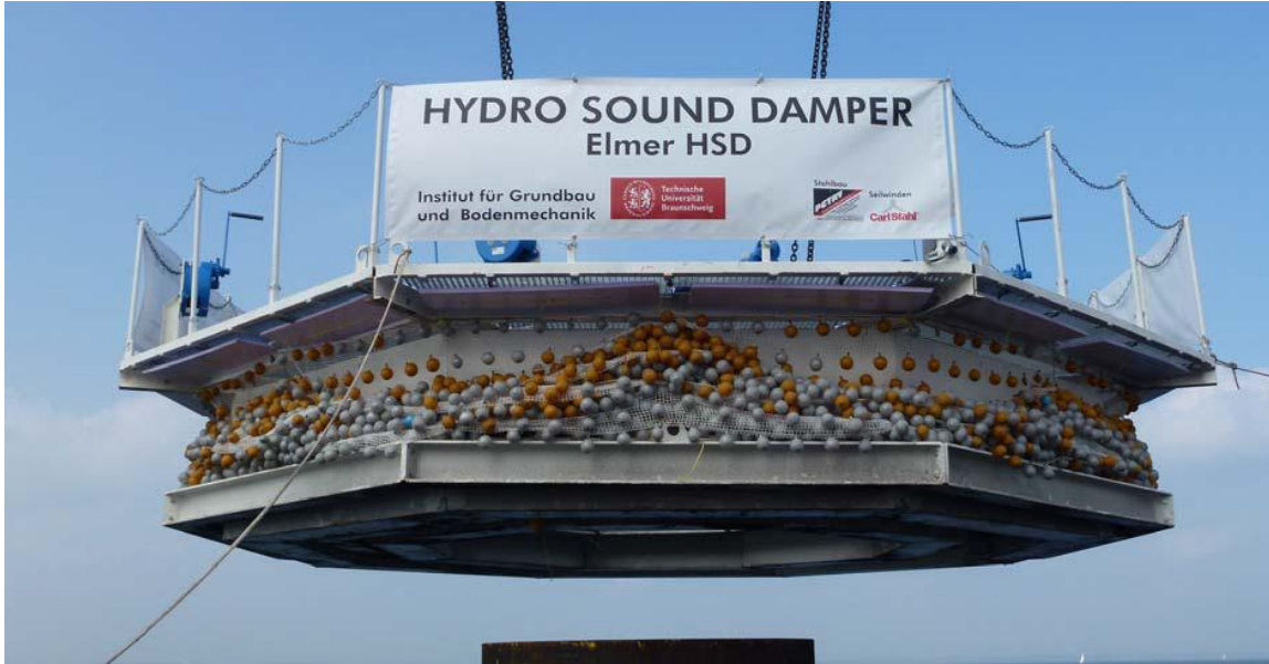
Figure 31: The entire HSD platform above the test pile (photo: Patrice Kunte)
