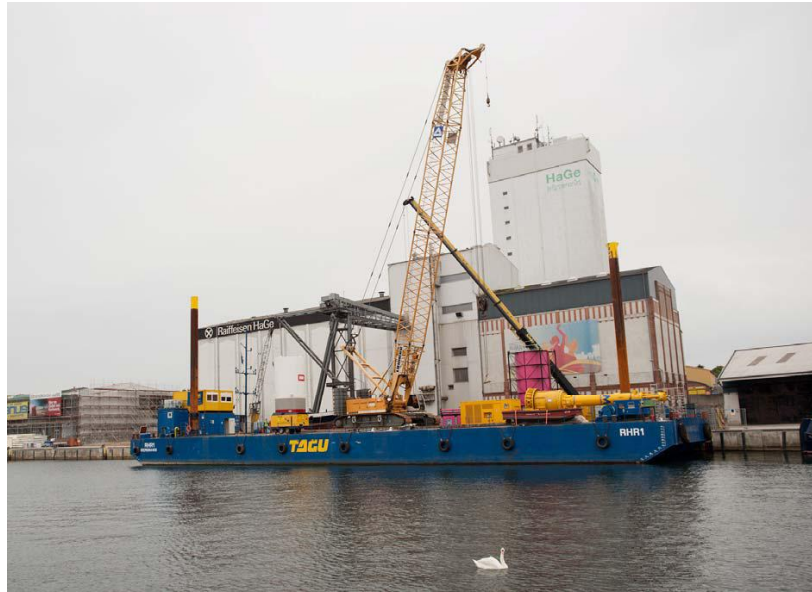
Figure 8: Stilt-mounted pontoon RHR 1 with equipment (photo: Patrice Kunte)
