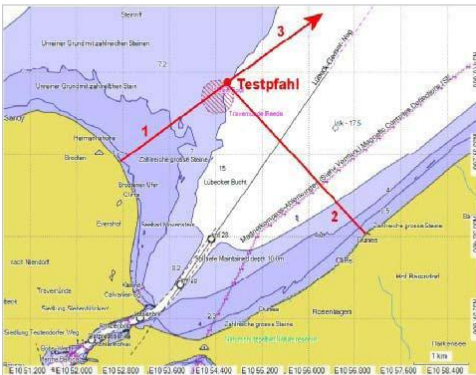
Fig. 2. Geographical position of the test pile. The red lines indicate the directions for which the noise propagation was calculated by way of example; see Sections 3 and 4.
