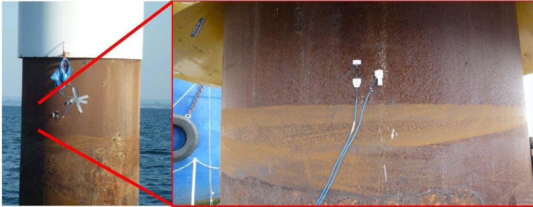
Figure 37: Measurement position of acceleration sensor (right) and expansion sensor (left) at the Brodten pile
