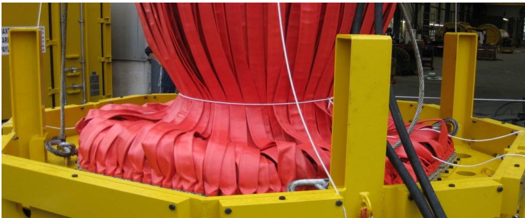
Figure 15: Close-up of the lower end of the NMS with the fire hose connections (photo: Patrice Kunte)
