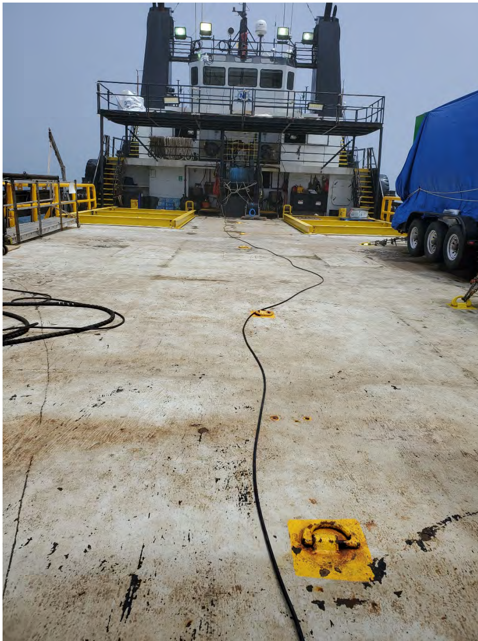
4) Deck cable runs from wheelhouse, across length of back deck, to tow cable.
